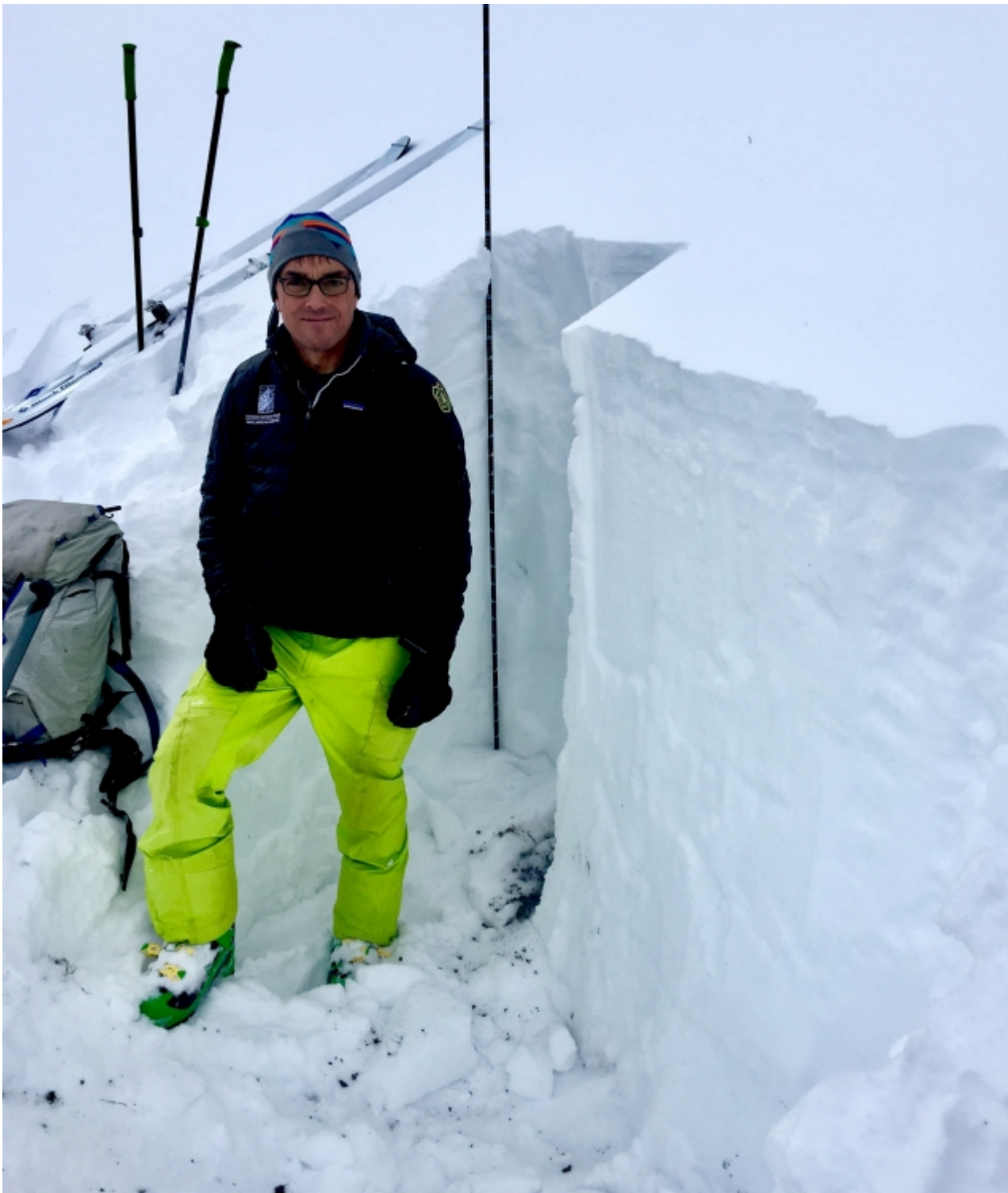
Doug stands in the a snowpit on a NE facing slope at 7,770 ft. on Mt Ellis. The snowpack is roughly 5' deep with no discernable weak layers. This is one of the best snowpacks we've seen on Mt Ellis in years. Photo: GNFAC
