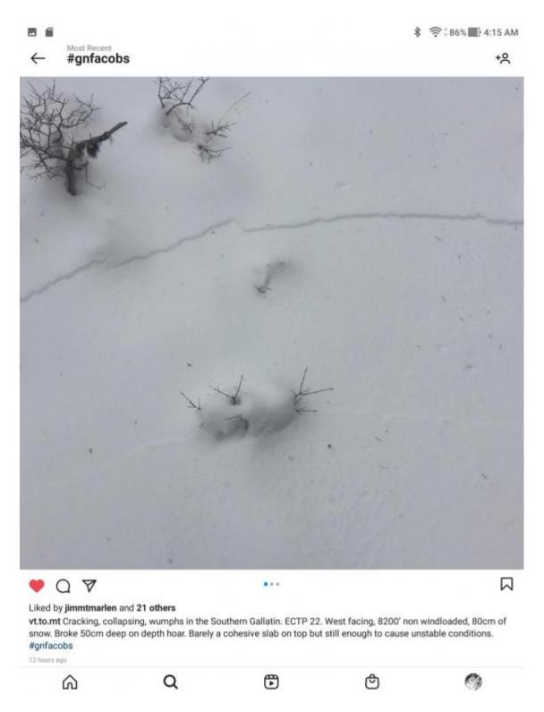
Cracking, collapsing, wumphs in the Southern Gallatin. ECTP 22. West facing, 8200' non windloaded, 80cm of snow. Broke 50cm deep on depth hoar. Barely a cohesive slab on top but still enough to cause unstable conditions.
