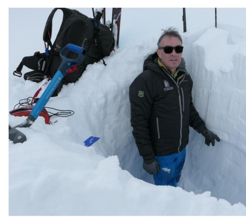
A 70 cm wind slab broke on the facets in our stability test (ECTP 21) and also in the avalanche. Photo: GNFAC
