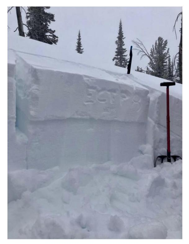
A layer of nsf's and surface hoar was failing ~10 inches deep producing easy ECTP's
