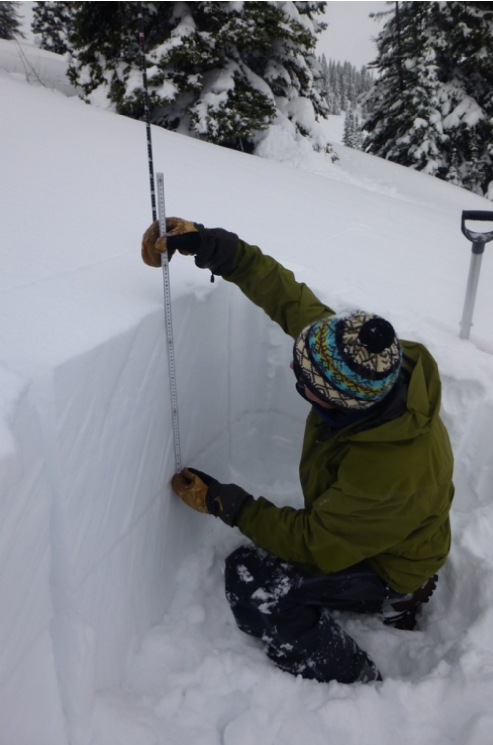
Karl Birkeland measures the 50cm slab sitting above the buried surface hoar layer. It propagated in 21 of 24 stability tests with ECTP12-14. Photo: GNFAC
