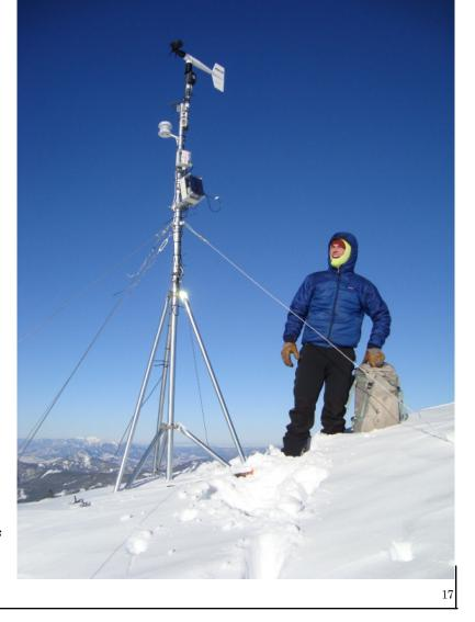
Mark Staples sets up the weather station near the summit of Flander's Peak in the Hyalite drainage.
